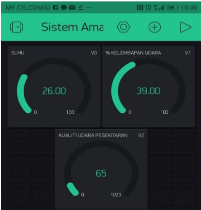
Figure 4: Temperature , air humidity and air quality reading from Blynk message
